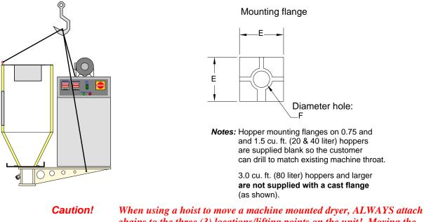
chains to the three (3) locations/lifting points on the unit! Moving the Dryer without the chains attached to all of the lifting points will cause the unit to become unstable and may cause damage to the Dryer and/or injury to personnel!
